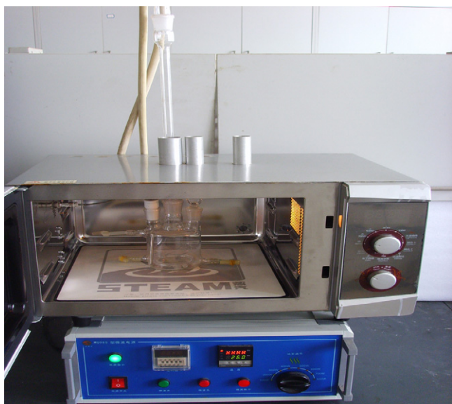
Fig. 1. The whole apparatus used in MW (MW)-enhanced and CH-enhanced \text{H}_2\text{O}_2 -based conditions.
